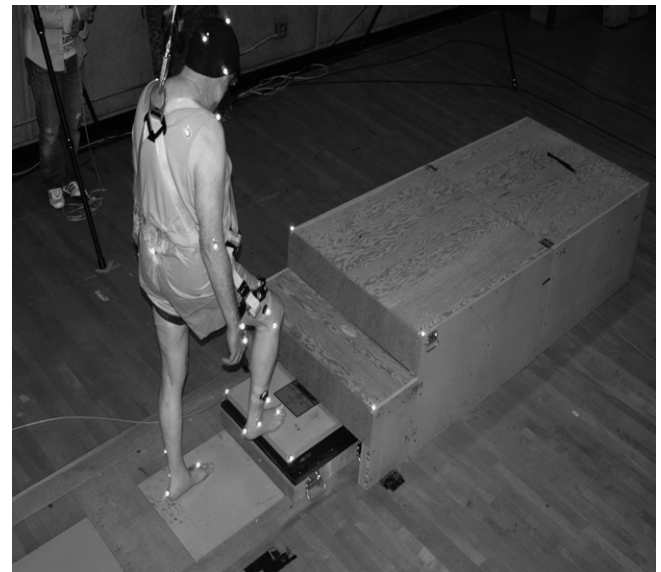
Fig. 3. A subject stepping onto the 3rd force plate which served as an independent first step of a 3-step staircase.
